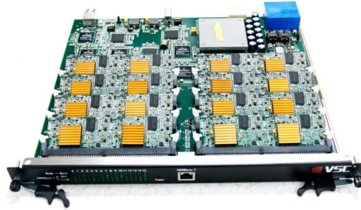
Figure A1: Accelerating cluster with 16 Zynq XC7Z030-3 SoCs.
